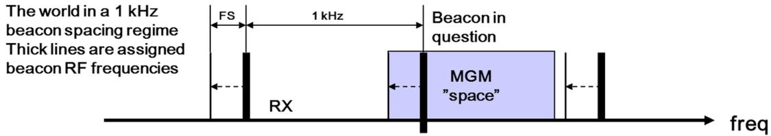
Should MGM be implemented on a beacon, a standard 1kHz tuning offset should be adopted as per the example in the diagram.
